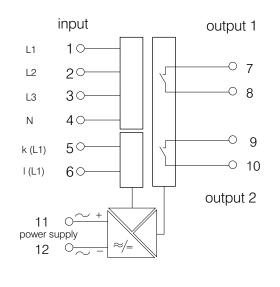
connection data: fine-wire 2,5 mm<sup>2</sup> single-wire 4,0 mm<sup>2</sup> max. voltage 250 VAC manner of fastening attachment rail NS 35 / 7,5 protection IP 20 weight approx. 200 g
