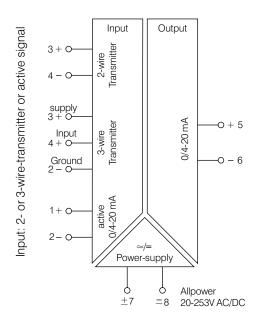
120 g weight protection: IP 20 manner of fastening: attachment rail: NS35/7,5; NS 32
